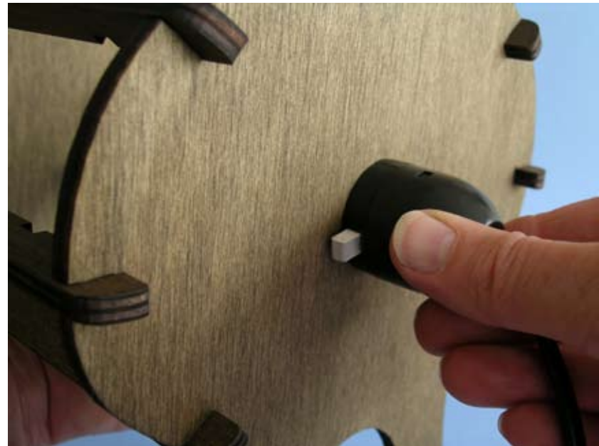
Fit the lamp holder through the hole in the rear.
