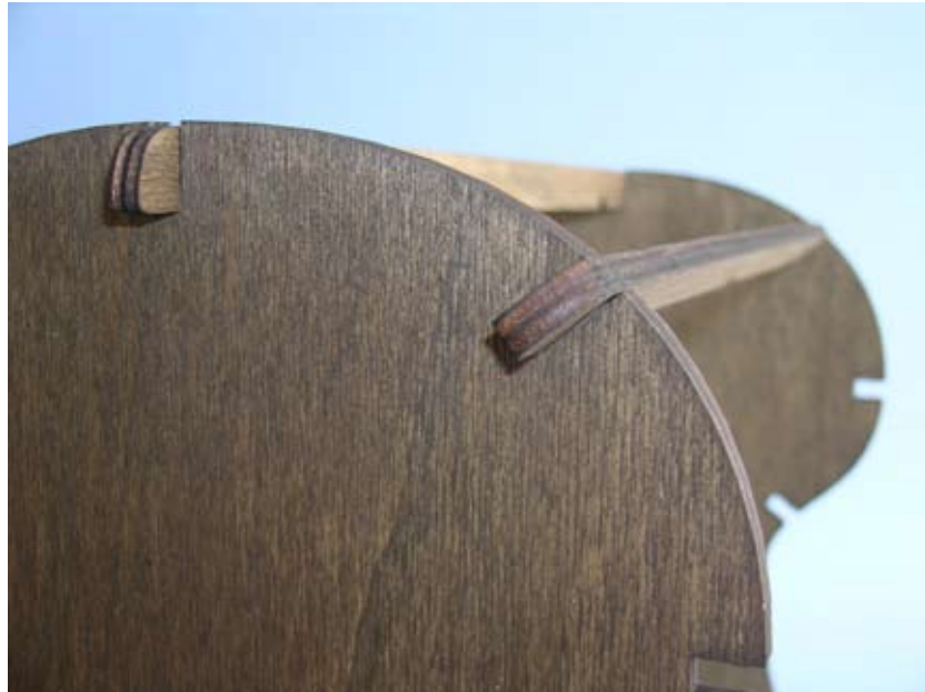
Make sure all the struts are in as far as they can go, so that the edges are flush with the front and back pieces.
